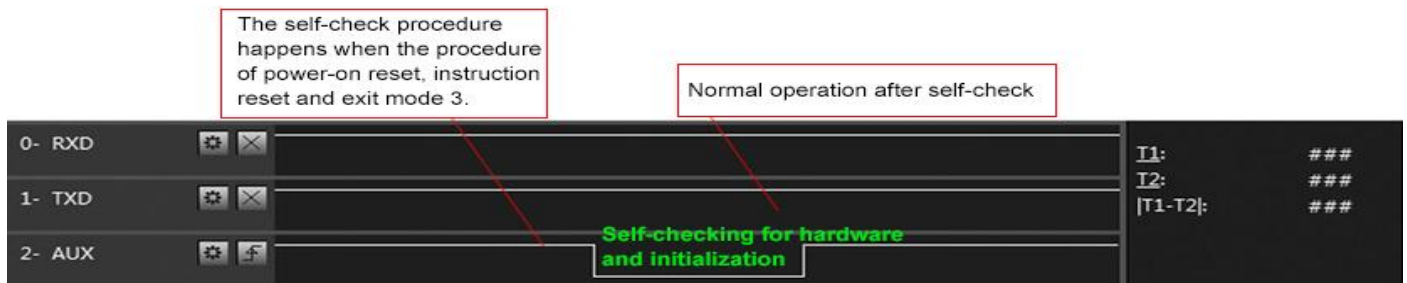
Timing Sequence Diagram of AUX when self-check
