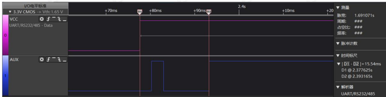
Figure 4 Power-on startup timing diagram
