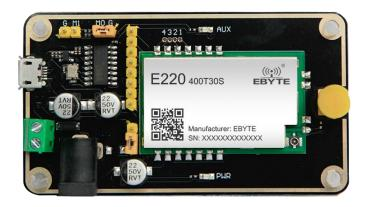
As shown above, connect to jumpers (5V power supply, mode 2), see function details from E22 UART module manual.
