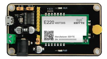
As shown above, connect to jumpers (5V power supply, mode 0), both EXX-XXXTBH-01 are configured this way, open serial port, for data TX and RX, and AUX indicator is blinking.
