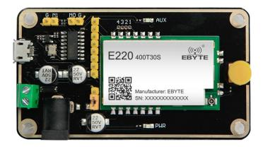
As shown above, connect to jumpers (5V power supply, mode 3), see function details from E22 UART module manual.
