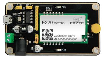
As shown in the figure, plug in the jumper (select 5V power supply, mode 3). For details, please refer to the corresponding serial port module manual.
