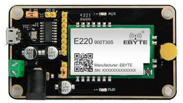
As shown in the figure, plug in the jumper (select 5V power supply, mode 1). For details, please refer to the corresponding serial port module manual.
