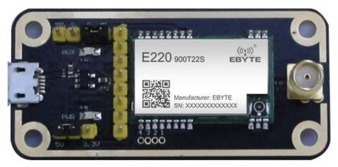
As shown in the figure, plug in the jumper (select 5V power supply, mode 1). For details, please refer to the corresponding serial port module manual.
