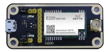
As shown in the figure, plug in the jumper (select 5V power supply, mode 2). For details, please refer to the corresponding serial port module manual.
