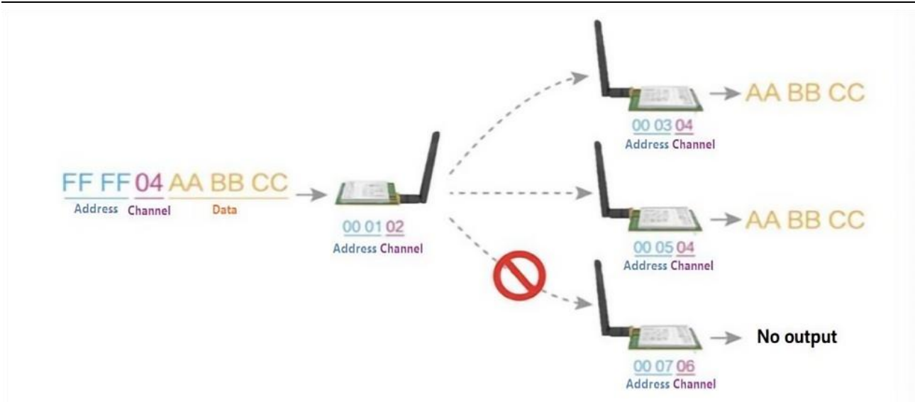
Fig. 2 Schematic diagram of fixed-point broadcast transmission
