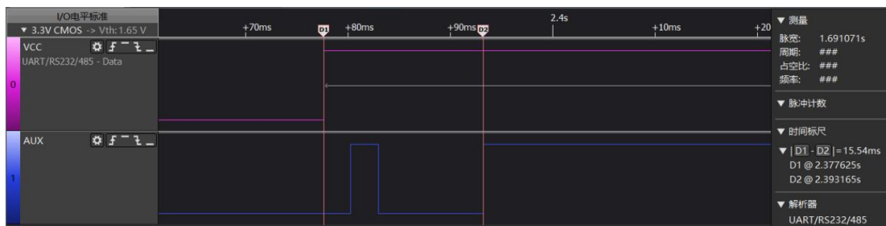
Figure 4 Power-on startup timing diagram
