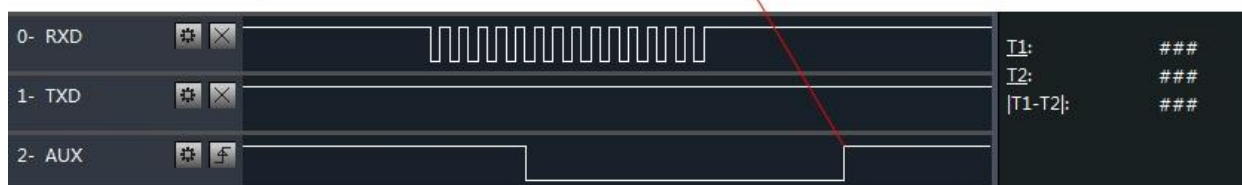
AUX pin timing diagram when the module receives serial port data.
