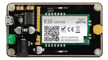
As shown above, connect to jumpers (5V power supply, mode 0), both E32-433TBH-01 are configured this way, open serial port, for data TX and RX, and AUX indicator is blinking.
