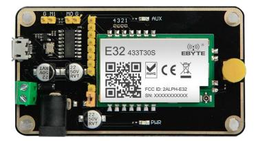
As shown above, connect to jumpers (5V power supply, mode 3), see function details from E32 UART module manual.
