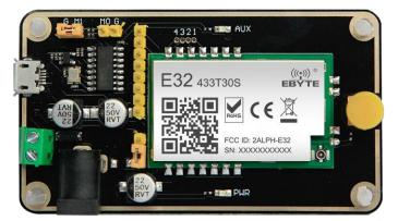
As shown above, connect to jumpers (5V power supply, mode 1), see function details from E32 UART module manual.
