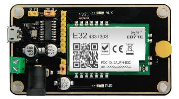
As shown above, connect to jumpers (5V power supply, mode 2), see function details from E32 UART module manual.
